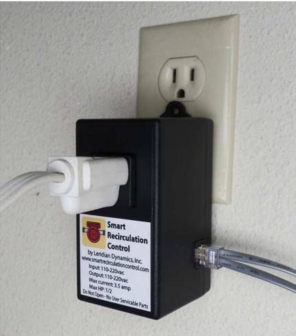
12. Plug the Smart Thermostatic Control into an electrical outlet and plug the recirculation pump into the Smart Thermostatic Control.
