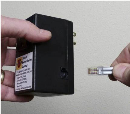
11. Plug the wiring harness into the Smart Thermostatic Control via the RJ-45 connector.
