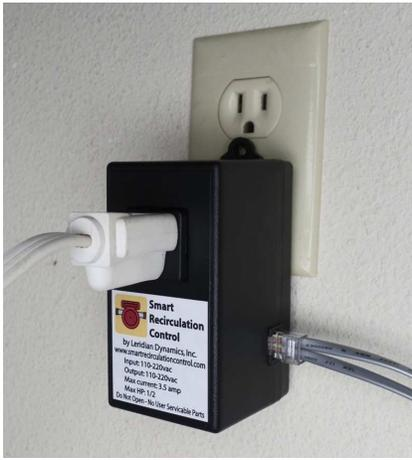
16. Plug the Smart Recirculation Control into an electrical outlet and plug the recirculation pump into the Smart Recirculation Control.
