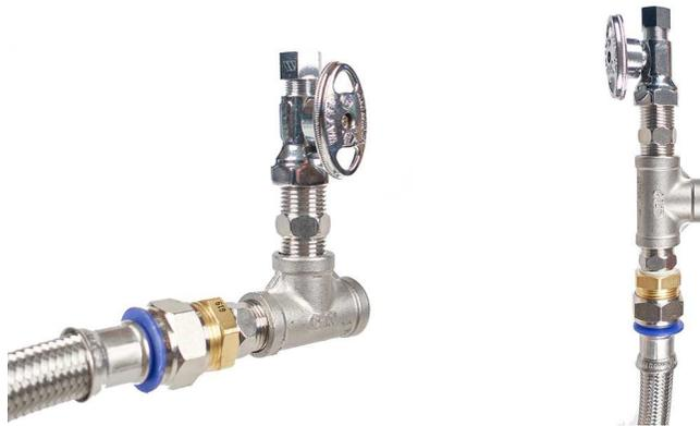
7. Once you know how the Tees are going to be installed and prior to attaching the Tees to the rough plumbing, attach the nipples to the correct ports on the Tees using PTFE tape and attach the shutoff valves to the nipples using PTFE tape. 4 to 6 wraps of PTFE is recommended for stainless steel.
